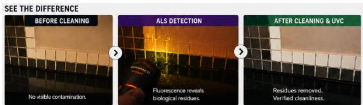
Figure 3. Evidence-based hygiene verification workflow. A surface that appears visually clean under conventional lighting often retains invisible biological residues. ALS inspection reveals fluorescent contamination hotspots. In the proposed localized workflow, the identified hotspot receives targeted UVC before physical cleaning; ALS reinspection then verifies whether fluorescent residue has been removed. Fluorescence indicates residual biological or
